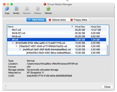
In all of these situations, from the point of view of the virtual machine, the virtual hard disk behaves like any other disk. While the virtual machine is running, there is a slight run-time I/O overhead because VirtualBox might need to look up sectors several times. This is not noticeable however since the tables with sector information are always kept in memory and can be looked up quickly.
